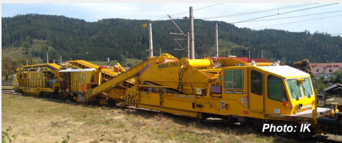
Photo 5. Ballast cleaning machine RM85-750
