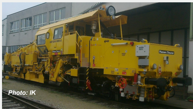
Photo 6. Ballast profiling machine USP 2010 SWS-U
