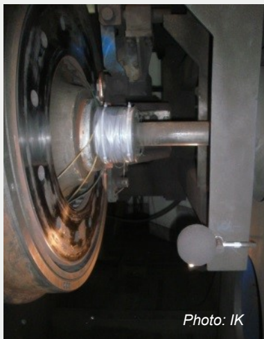
Fig. 3 Location of a microphone for measuring noise in the test cabin
