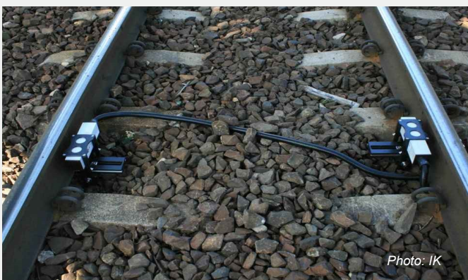
Fig. 2. Measurement antennas mounted to the rails
