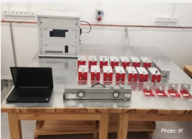
Fig. 1. Stand for testing immunity to conducted disturbances, induced by radio frequency fields
