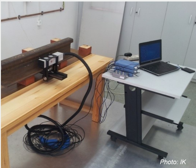
Fig. 1. View of the magnetic field test stand (laboratory)
