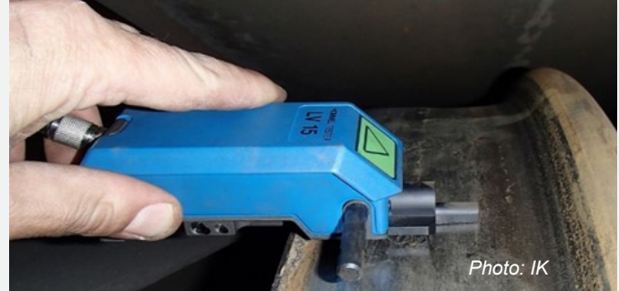
Fig. 1. Measurement of the running surface roughness of a railway wheel (the author's own material)
