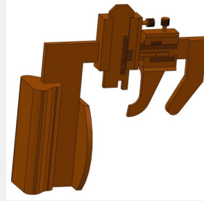
Fig. 2. Callipers for measuring the wear of wheel running surface
