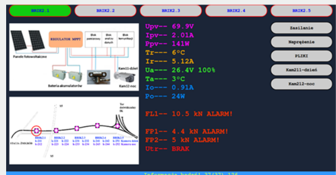
Fig. 2. The view of the information panel in the state of alarms
