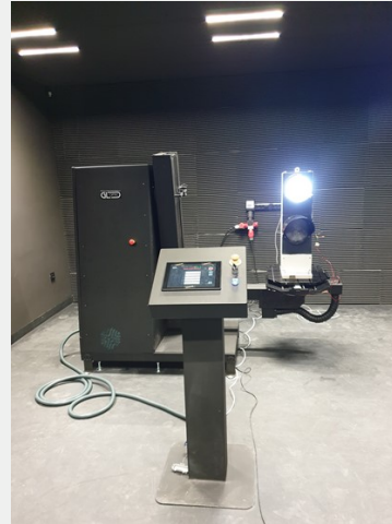
Photo 1. Goniophotometric test stand with mounted dwarf signalling device for testing
