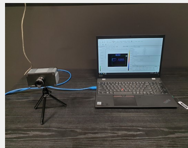
Photo 2. Measurement stand for measuring the luminance of a luminous surface
