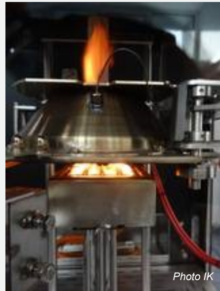
Photo 1. Cone calorimeter test according to ISO 5660-1
