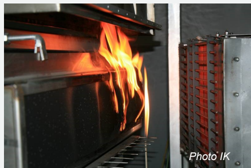
Photo 2. Flame spread test in vertical configuration in accordance with ISO 5658
