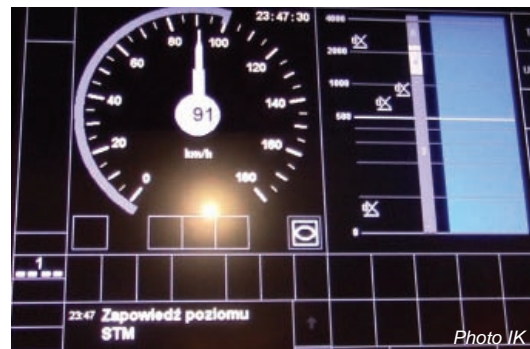
Figure 1. Example of DMI monitor imaging during ongoing tests [Photo: Author]
