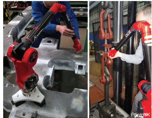
Fig. 3. Measurement of bogie frame and screw coupling with measuring arm
