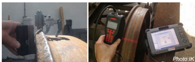
Fig. 2. Measurement of a defective wheel set
