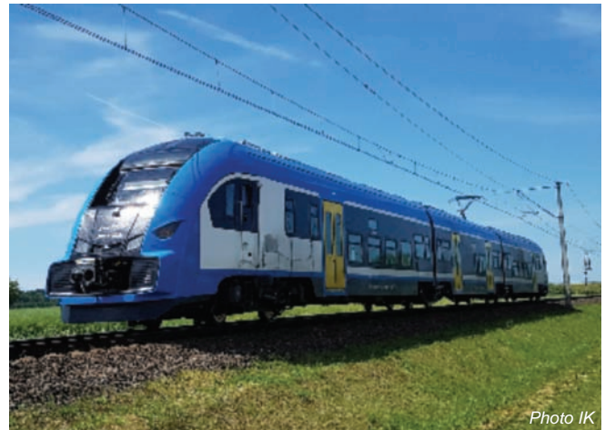
Fig 2. EMU during functional tests of Eurobalises
