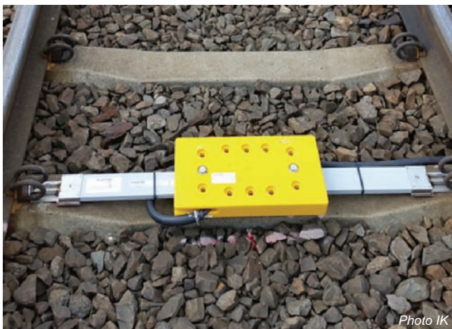
Fig 1. Eurobalise mounted on the rails
