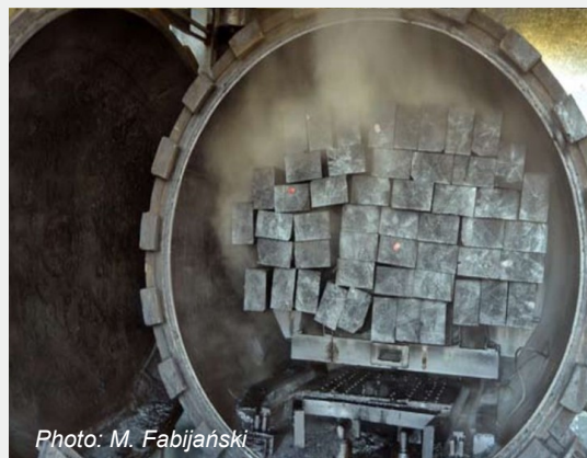
Fig. 2. Impregnation cylinder used for impregnation of wood material by the Rüping method
