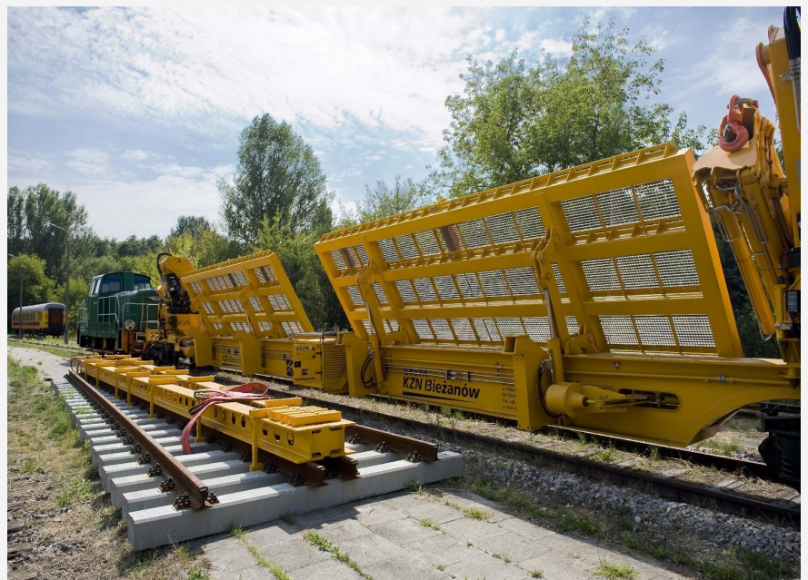
Photo 2. Preparation of a turnout to be loaded onto the wagon
