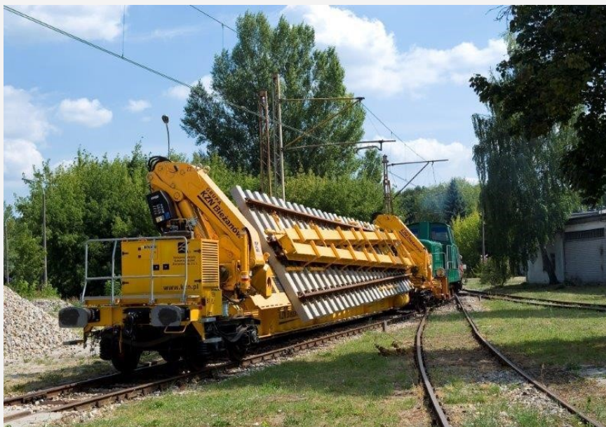
Photo 4. Wagon KZN01A type loaded with a turnout
